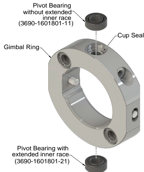
Figure 6.10—Gimbal Pivot Bearing Replacement
