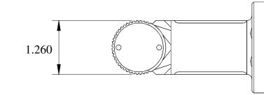
Figure 6.1—Hiac and Tool Center Point (TCP) Dimensions
