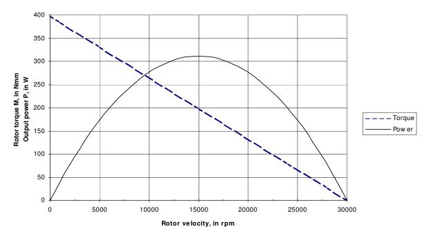
Figure 5.2—Theoretical Calculations, Hiac Output Torque and Power
